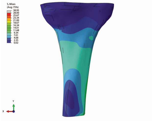
FIGURE 3. Variation of the equivalent von Mises stress for tibia in case of proximal resection at 1.5^\circ angle (anterior) in sagittal plane
